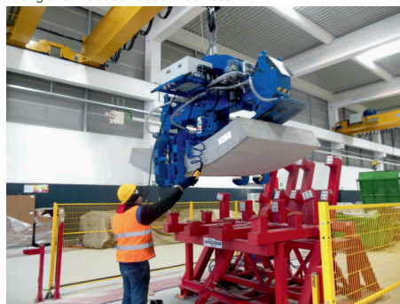
Tilting and Intrados Vacuum devices
