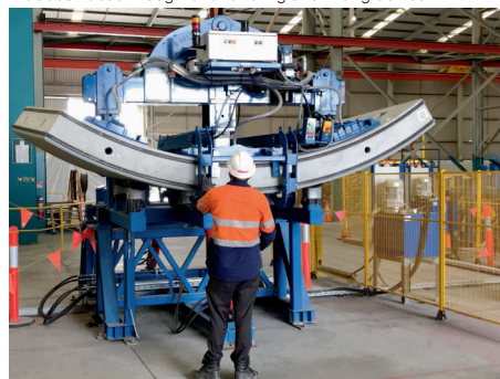
Intrados vacuum segment handling and Tilting device
