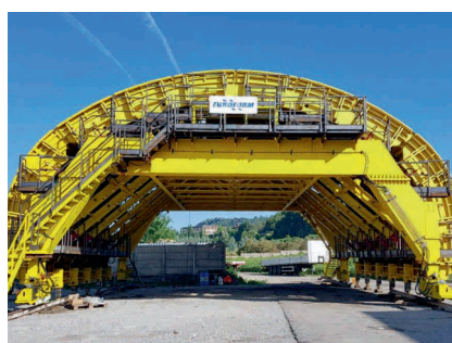
Main tunnel formwork
