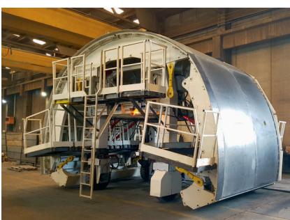
Cross Passage formwork
