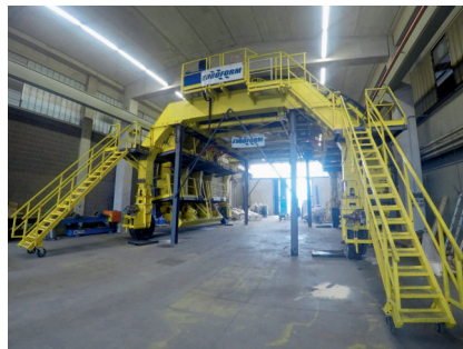
Ramp tunnel formwork
