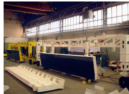
Ramp tunnel kerb formworks
